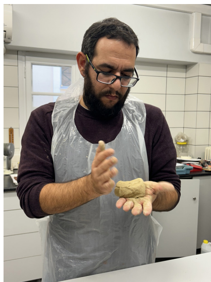
Rafael working with clay from Oued Beht to make briquettes
